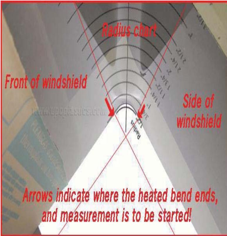
To measure the radius curve, cut this scale from the page starting at the 2" radius scale mark.
