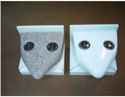
The suicide prevention 4" spread faucet is basically a Chicago meter type faucet that is encase in Corian material. It is designed so that a patient cannot tied anything to it and use it as a hanging point. The fixture sits on the top of sink and the rear of the faucet extends to either the backsplash or the wall. (See attachment)
